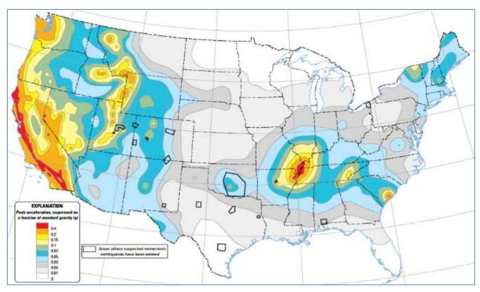
Figure 11-6. Peak Horizontal Acceleration with 10% Probability of Exceedance in 50 Years
